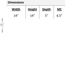
A 4" octagonal junction box should be used for installation MC = Mounting Center, located at center of fixture unless noted otherwise
