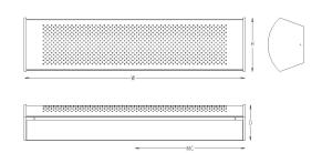
A 4" octagonal junction box should be used for installation MC = Mounting Center, located at center of fixture unless noted otherwise
