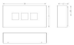
A 4" octagonal junction box should be used for installation MC = Mounting Center, located at center of fixture unless noted otherwise
