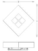
A 4" octagonal junction box should be used for installation MC = Mounting Center, located at center of fixture unless noted otherwise
